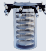
8-12 Port Acrylic Drying Chamber with Manifold and complete valve flask attachment
